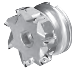
Steel base body with IC Cutting edge setting 5° 90° cutting up to 7mm Tightening torque 1,20 Nm
