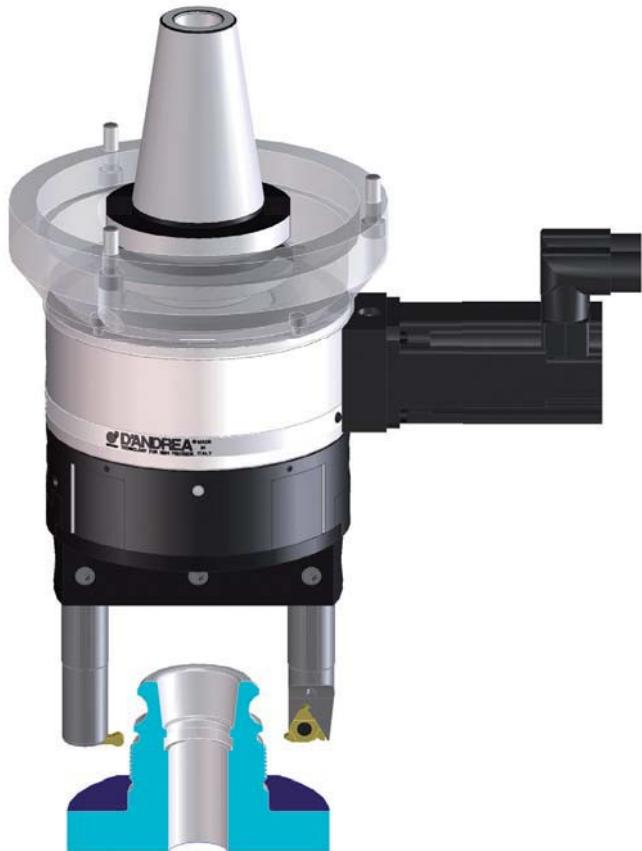
TA-TRONIC boring and facing heads can be manually or automatically applied on small boring machines, machining centres and special machines. Connection with the machine tool spindle occurs through a cone for the rotation of the rotating head and a flange for fastening the fixed body on to the fixed part of the machine. For lighter tasks a simple anti-rotation pin may be used. Two possibilities are available for the control unit of the TA-TRONIC head:
